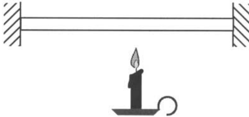
Figure 9.2. A clamped beam subjected to thermal stress.
